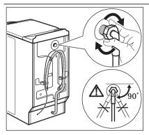
Connect the hose to the appliance. Loose the ring nut to set it in the correct position.
